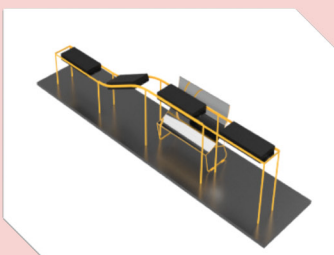
Solar parabolic trough-based fish dryer
